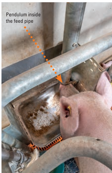
Sensor-controlled: sow actuating pendulum inside the pipe
