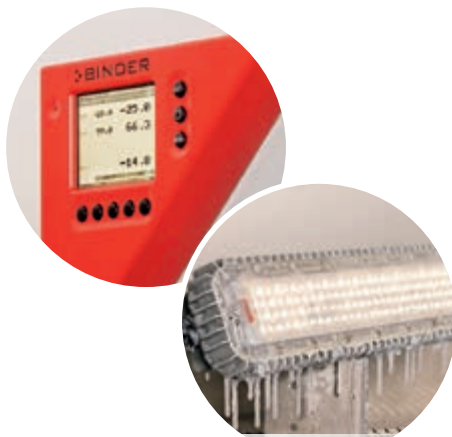
ZeusLED ceiling lamp, tested under temperatures of -25 °C
