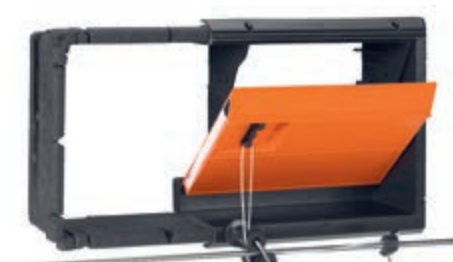
CL 1211/F Anti-Freeze – flange inlet with the best possible insulation of inlet flap and frame for very cold regions with temperatures below -25 °C: nearly no formation of ice at the inlet
